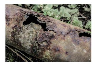
The corrosion of metal pipes can be due to galvanic currents or water with low salt content, but in any case it is crucial for the exchange of free electrons from metal to water.
