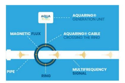
AquaRing® emits complex multi-frequency signals on water distribution pipes (AquaRing® patent pending signals). This process follows the transformer principle: the pipes, with the ring and the water in them, represent the secondary coil.
